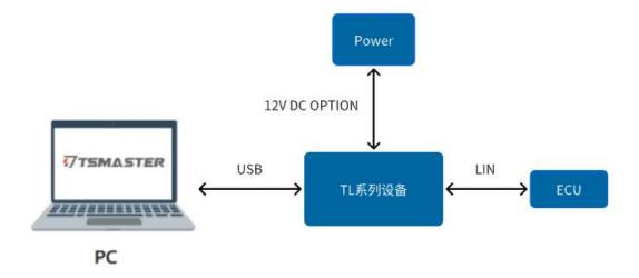
Connect the TL series device to a computer via the USB interface and connect the LIN communication interface to the ECU. Optionally, power the device using a DC power supply. Then on the PC side, users can control the LIN communication between the device and the ECU with the powerful TSMaster software.
