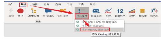
Step5: Start the connection, start the FlexRay network, when you can hear the TC1034 relay sound. Channel FR 2A and 1A can be observed in the FlexRay message.
