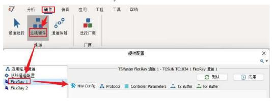
FlexRay The hardware configuration is divided into HW Config, Protocol, Controller Parameters, Tx Buffer, and Rx Buffer.
